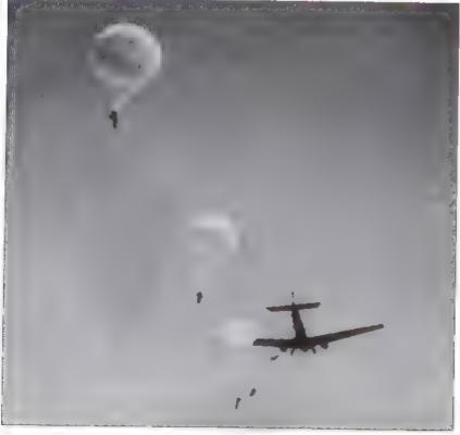
ABOVE The moment of truth. The static line has just reached full stretch and the paractiute pack of the lower figure, failing in the recommended spread-eagled posture, is just coming open while a second man vaults from the Ju 52's door.
